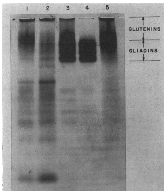
FIG. 1. Starch-gel electrophoretic patterns of protein fractions obtained by ultracentrifugation and solubilization in 70% ethyl alcohol of the pH 4.7 soluble gluten. The patterns represent: insoluble in 70% ethyl alcohol (glutenins, pattern 1), 100-5C glutenin, centrifugate from 100,000 x G for 5 hr. (pattern 2), 100-5S supernatant from soluble gluten after 100,000 x G for 5 hr. (pattern 3), soluble in 70% ethyl alcohol (gliadins, pattern 4), insoluble in 70% ethyl alcohol from 100-5S (100-5S glutenins, pattern 5), Ref. 3.
